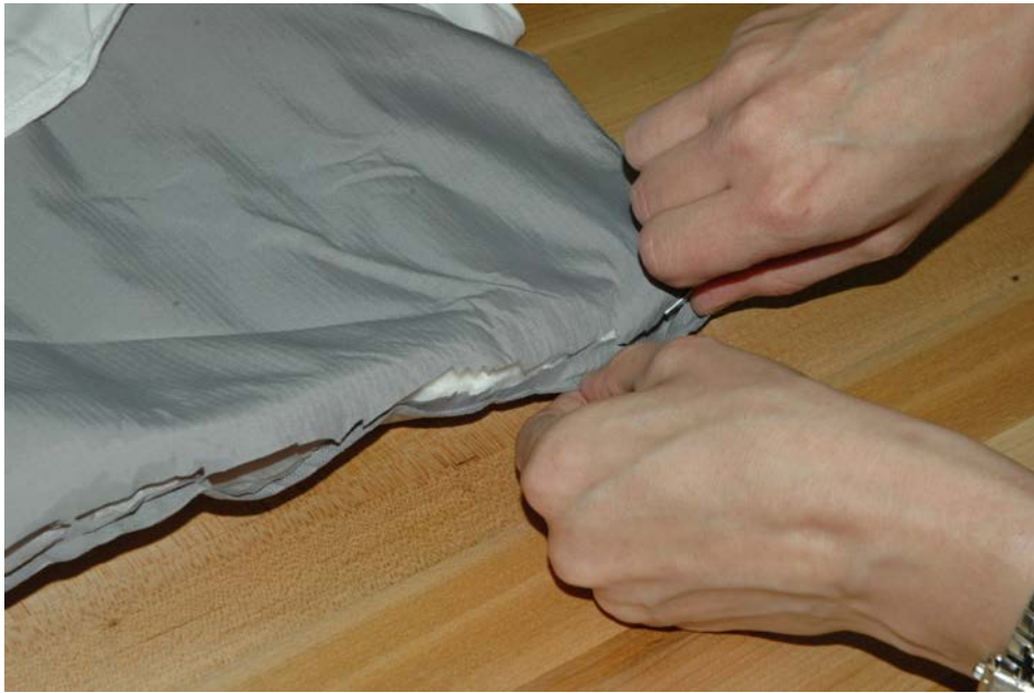
Figure 13: Completion of slit in bottom of armor panel cover.
