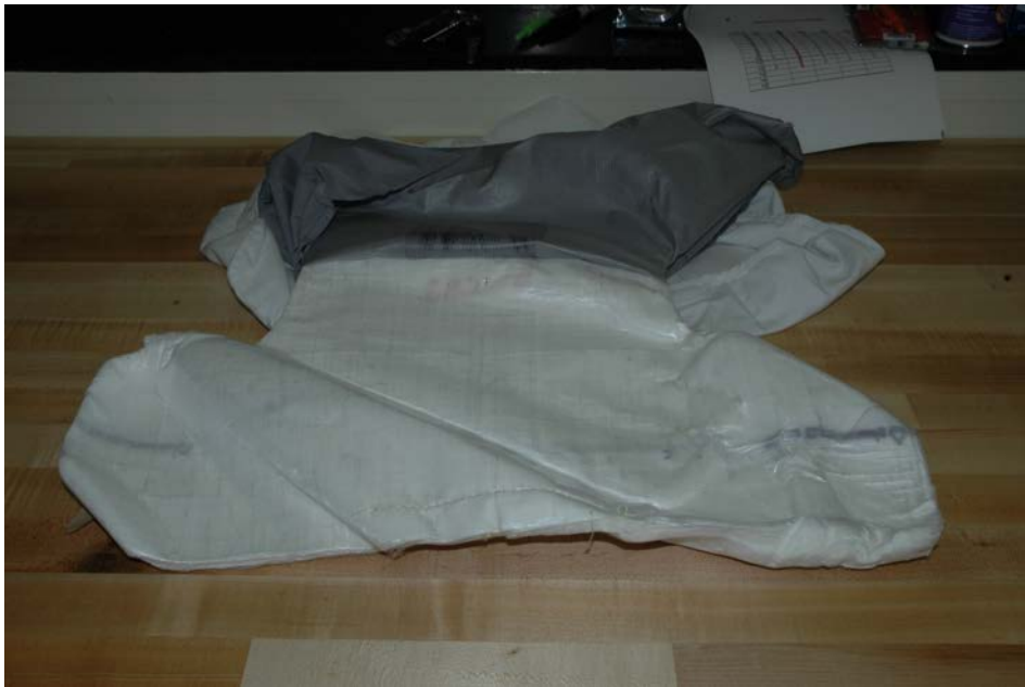
Figure 14: Armor panel with panel covering material folded back to allow access to ballistic package (so as to preserve original orientation of ballistic package within the armor panel cover). Note that the armor panel was not removed from the panel covering material.
