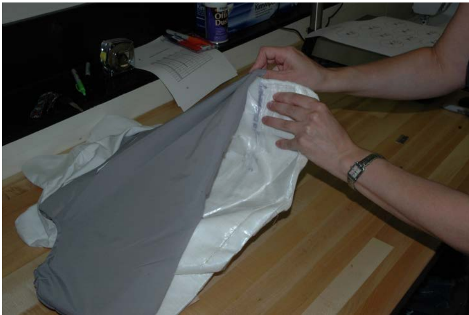
Figure 16: Reinsertion of the armor panel in the armor panel cover, preserving original orientation.
