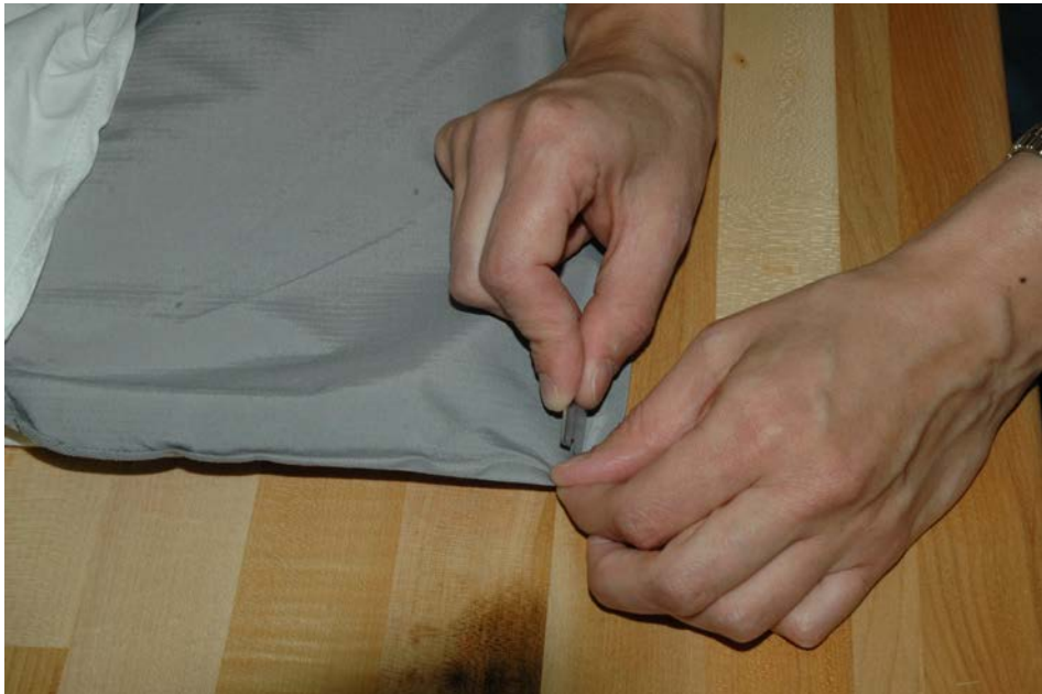
Figure 10: Use of a razor blade to to slit just the bottom of armor panel cover.
