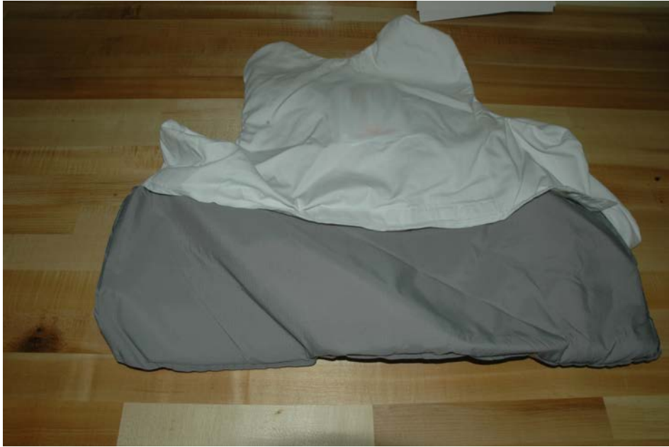
Figure 9: Armor panel prior to removal of armor panel cover.
