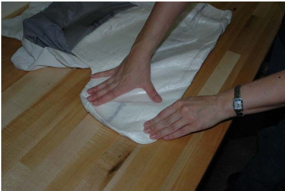
Figure 15: Use of flattening to press out additional wrinkles in the ballistic package.
