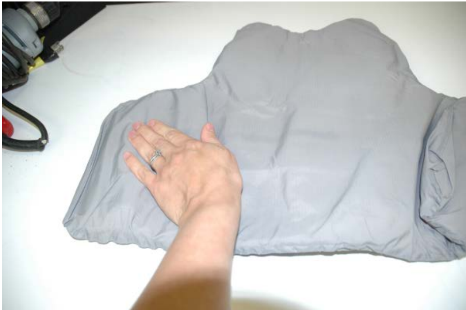
Figure 4: Demonstration of technique for unfolding and flattening armor panels.
