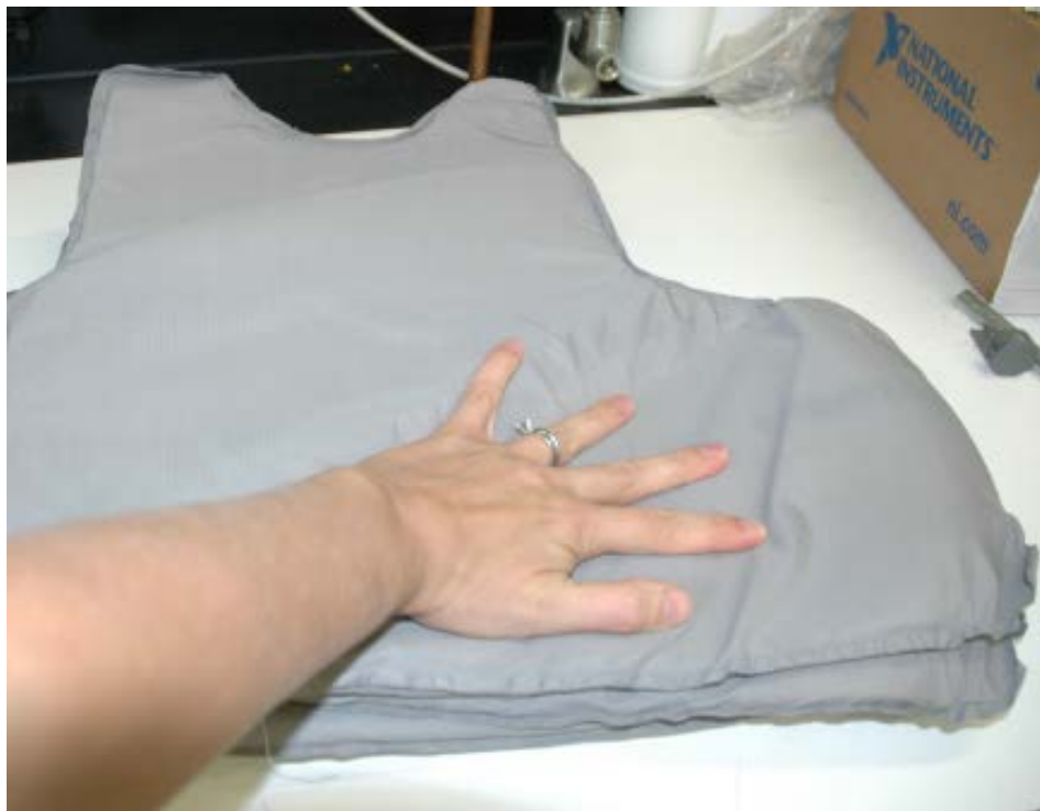
Figure 7: Stacking of flatter armor panels on top of wrinkled armors to assist in pressing out wrinkles.
