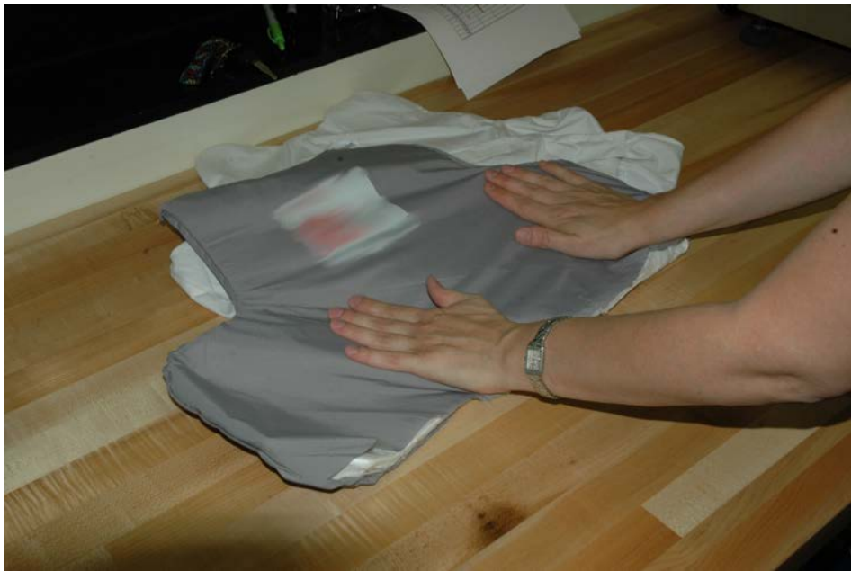
Figure 17: Smoothing and flattening of armor after reinsertion into the armor panel cover.
