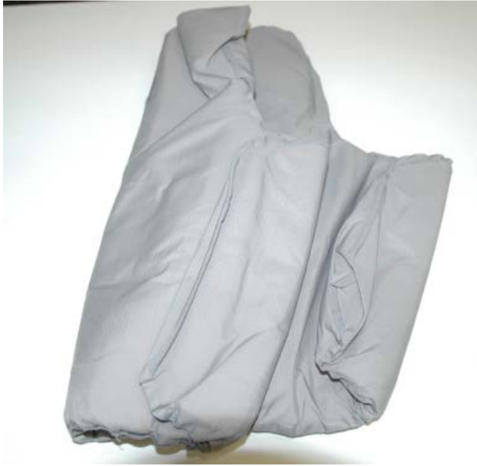
Figure 3: Folded and wrinkled armor panel after removal from tumbler.
